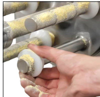
Magnets are cleaned completely outside the product zone.
