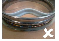
All care must be taken to ensure that the circumference of the head after fitting and welding remains the same size as supplied, to ensure fitting tolerance of the connector.
