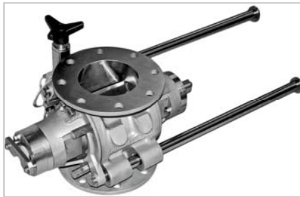
RV's with slide rails are available in 6 sizes covering a capacity range of the rotor from approximately .09 to 2.05 CFR at 100% filling.
